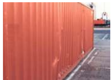
23 Dented external side panel.
