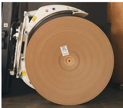
A 5° forward tilt ensures that the short arm pad is under the paper roll and the long arm pad is over the top. Source: Cascade
