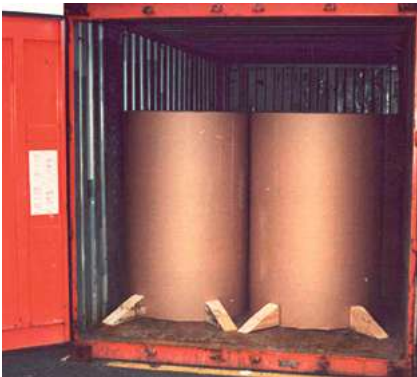
✗ Insufficient blocking / bracing. Source: FMS 'Use No Hooks'
