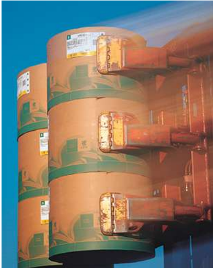
Multiple rolls of graphic paper can be moved with multi clamp trucks. Source: UPM
