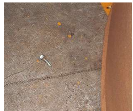
✗ Potential roll end damage source — loose screw. Source: IF P&C
