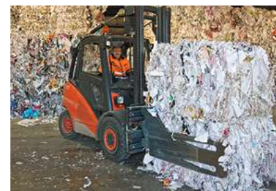
Dedicated clamps are required to handle RCP bales. Source: UPM
