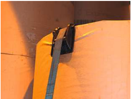
✗ This photo shows correct edge protection but the wrinkles on the wrapping shows poor practice caused by the lashing down force being too high. Source: Stora Enso
