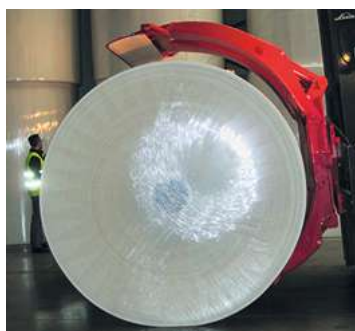
Short arm should be against the floor when lifting a roll from the ground. Source: Bolzoni Auramo
