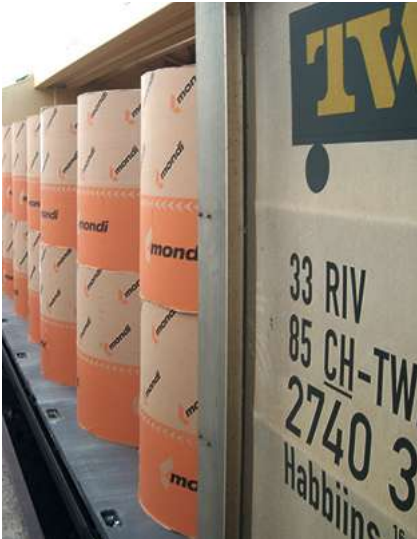
Habbiins rail waggon loaded with standing rolls. Source INTAKT
