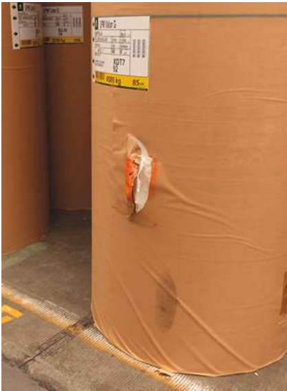
Side damage (belly) caused by a clamp truck's counter weight. Source: UPM
