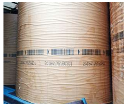
Rolls showing condensation. Source: Stora Enso
