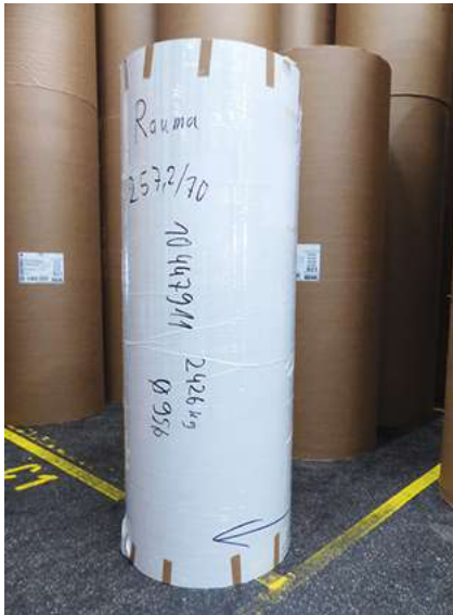
Always re-wrap partly used rolls in a suitable protective material. Source: UPM
