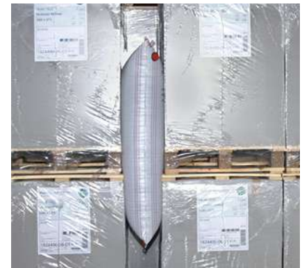
Correctly placed airbags reduce damage by preventing cargo moving into gaps. Source: INTAKT
