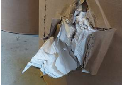
Side damage from poor clamping. Source: UPM
