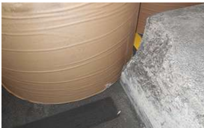
Roll damaged from collision with a pillar. Source: IF P&C
