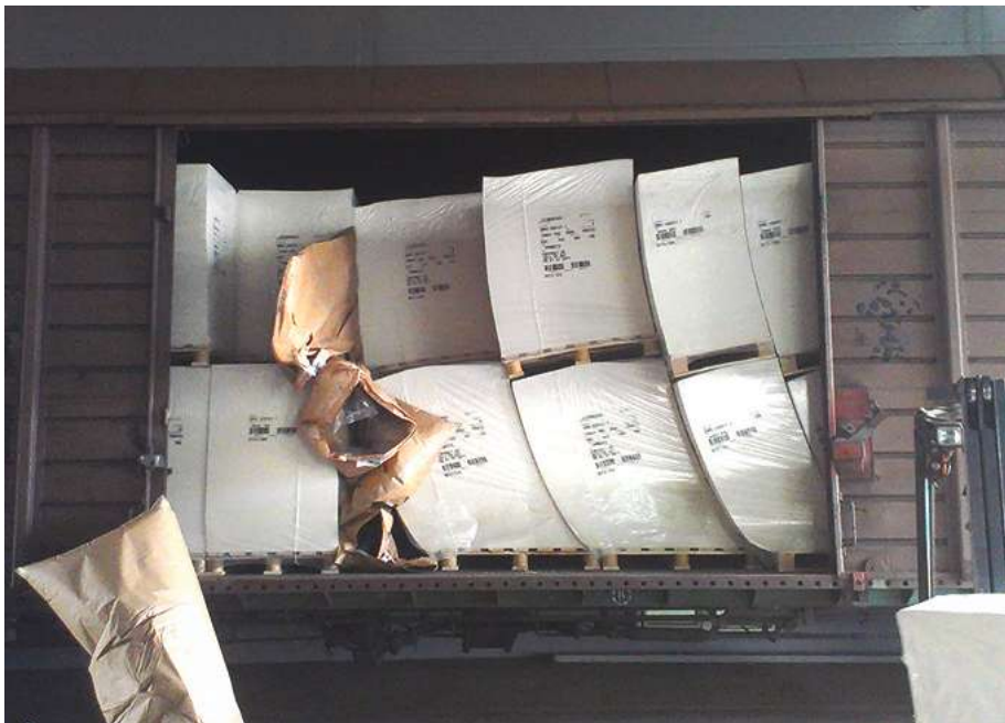
Stacked sheet paper tends to tilt or move within the smallest cargo gap when subjected to maximum impacts (sharp braking of a truck, railway shunting, or bad weather at sea). Stora Enso
