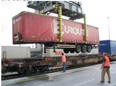
✗ This photo shows two bad safety practices (1) staff not wearing hard hats, (2) a person under a suspended load. Source: INTAKT
