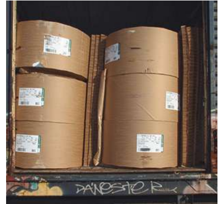
Dunnage used between rolls to reduce shifting of standing rolls. Source: INTAKT
