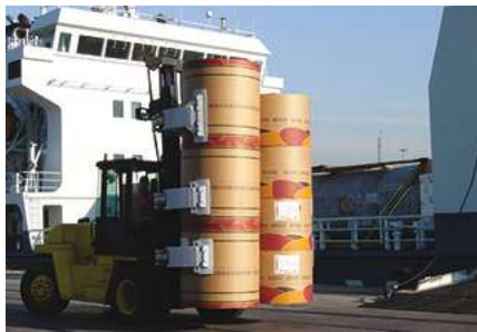
Rotating clamps for handling either jumbo rolls or up to three rolls for loading and unloading ships, rail wagons or trucks. Sources: (left) Bolzoni Auramo, (right) Cascade
