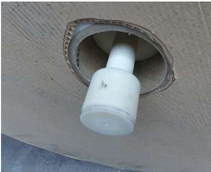
Device used to test core deformation. Source: UPM
