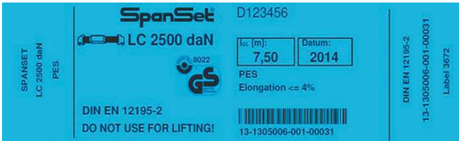
Typical content of webbing strap label, marked in accordance with EN 12195 2. Source: SpanSet/CEPI
