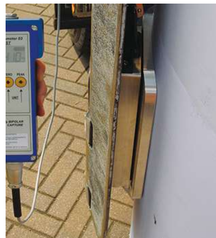
3: Test pad electronic measurement device uses highly accurate weighing cells mounted on a portable aluminium frame. The pad is put between the contact pad and the paper roll and when the clamping arm is closed, the test pad display shows the clamping force. For a split arm clamp, multiply the result with the quantity of split arm sections. This device is suited for quality control supervisors and service staff. Source: Cascade
