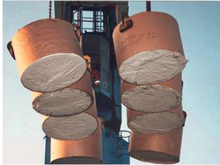
Eccentric load. Source: FMS 'Use No Hooks'
