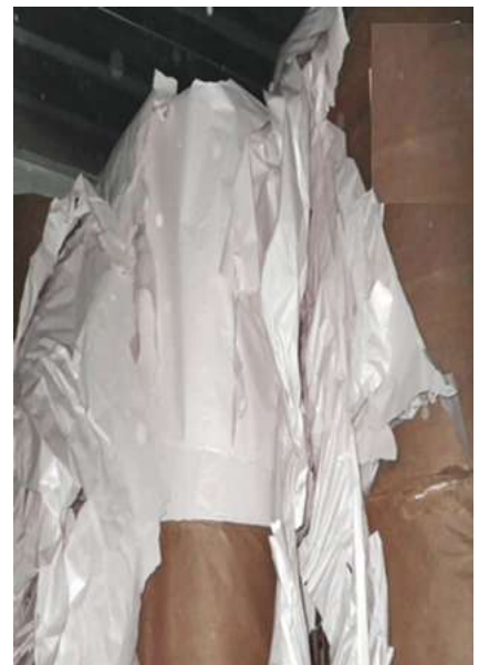
Severe chafe damage from excessive rail transport vibration. Source: Idealliance
