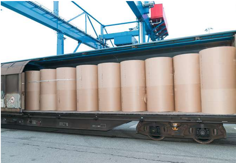
Standing rolls loaded in rows on anti-slip material. Source: INTAKT.
