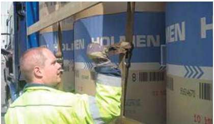
Heavy-duty ratchet for tie-down lashing. Use lashing straps with min. 4000 kg (8818 lbs) breaking strength. The recommended standard minimum to maximum pre-tension force is between 400 to 500 daN (899-1124 lbs). Source: Holmen
