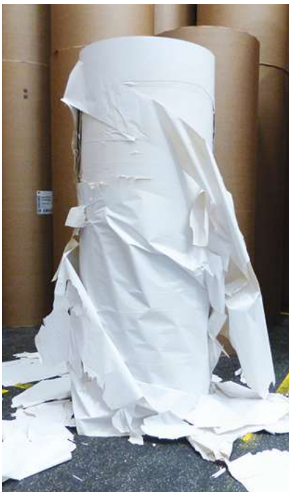
X Loose paper from unwrapped part rolls are a fire risk. Always rewrap rolls. Source: UPM
