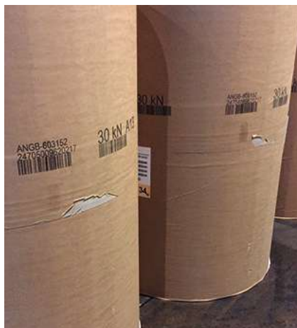
Belly wrapper damage. Source: Stora Enso
