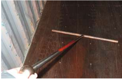
Tool to detect protruding screws is particularly useful in poor light conditions. Source: UPM
