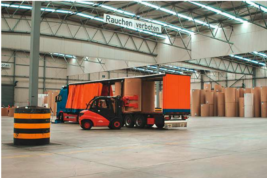
Truck loading inside warehouse, note protection around pillar. The roll should be clamped in the middle, not at the bottom. Source: 'FMS Use No Hooks'
