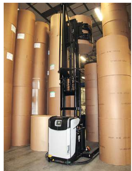
AGV automated roll handling. Source: KBA
