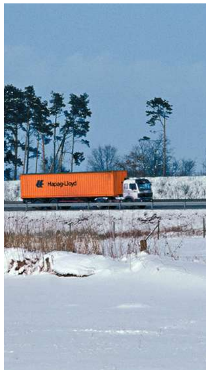
The paper on this truck was loaded at the mill at 50% RH at 23°C, during transportation the temperature fell to -10°C (14°F). Condensation will be formed unless it is correctly conditioned at its destination. Source: Hapag-Lloyd.
