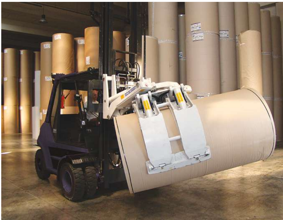
Horizontal paper rolls can also be handled with tine clamps. Source: Bolzoni Auramo
