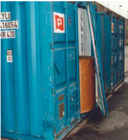
Container door damaged by cargo within. Source: FMS 'Use No Hooks'
