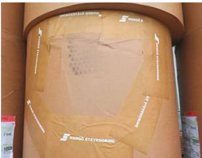
Rolls shifted from continuous brief impacts during rail or sea transport. Source: Mëtsa Board
