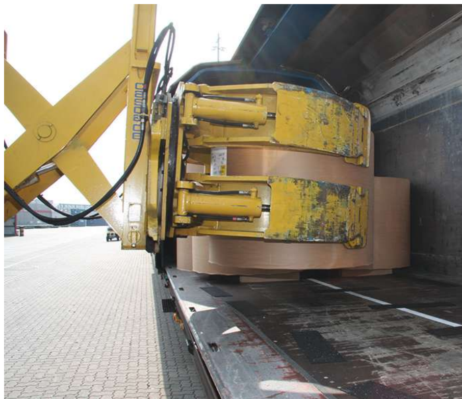
Load extender placing rolls on anti-slip material. Source: INTAKT
