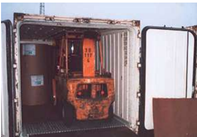
Containers impose height and weight limits on lift trucks.
