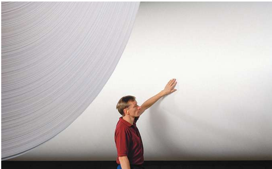
Paper machines manufacture very large tambours —also known as machine, jumbo or mother reels. Source: UPM
