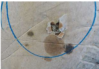
End damage from debris in floor. Source: UPM
