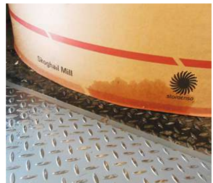
Contamination damage visible on wrapper. Source: Stora Enso
