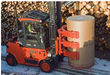
Rotating clamps for handling either jumbo rolls or up to three rolls for loading and unloading ships, rail wagons or trucks. Sources: (left) Bolzoni Auramo, (right) Cascade
