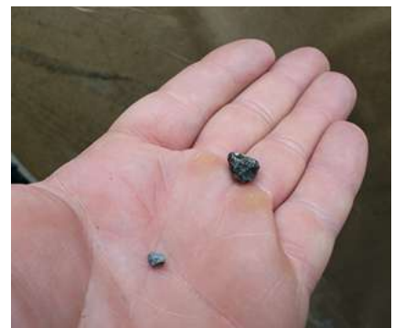
✗ Potential roll end damage source — gravel. Source: UPM
