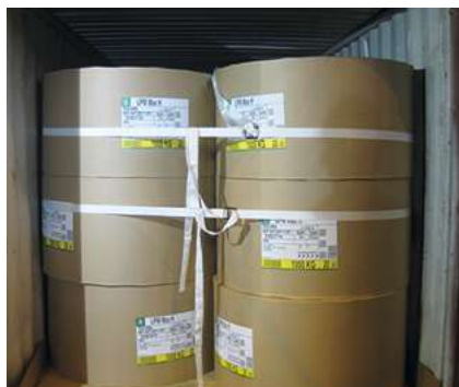
Cargo is secured with horizontal belts. The three tiers of rolls are secured with two belts, around the second and third tiers. Source UPM
