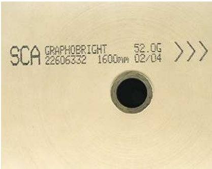
Ink jet printing on roll end shows roll number, weight, unwind direction and mill splice position. Source: WOCG/icmPrint
