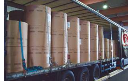
X Use straps and edge protectors to secure the rolls — edge protectors are missing in this photo. Source: Stora Enso
