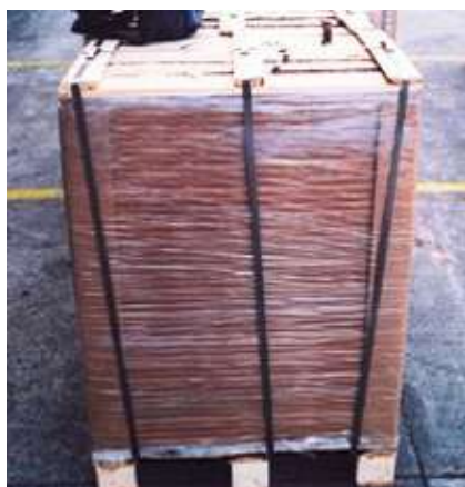
Pallet with paper in sheets with quintuple strapping. Source: FMS 'Use No Hooks'
