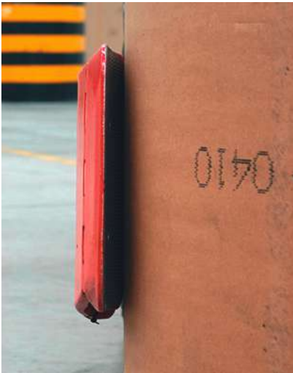
Gap between contact plate and roll. Possibly caused by incorrect position of clamp arms or too small clamp arms. Source: FMS 'Use No Hooks'
