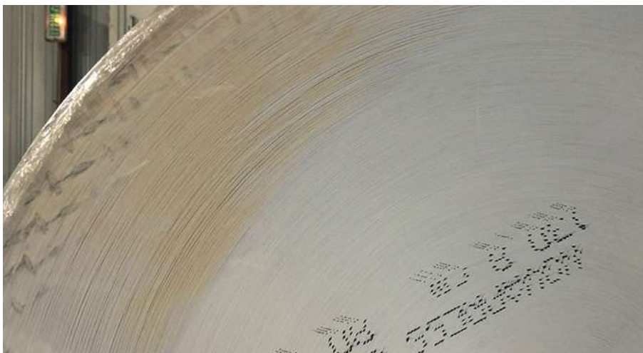
Roll with about 20% water damage. Source: Stora Enso
