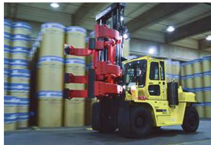
Non-rotating multiple paper roll clamps: Sources: (left) Bolzoni Auramo, (right) Cascade.
