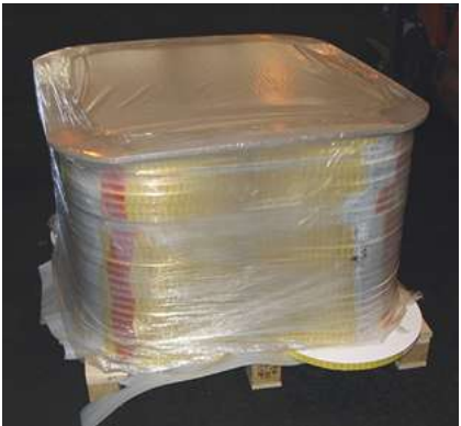
Slipped cargo unit. Source: FMS 'Use No Hooks'
