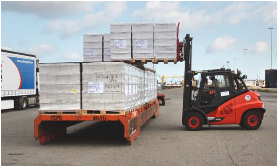
Plywood boards must be used between layers of pallets. Source: INTAKT
