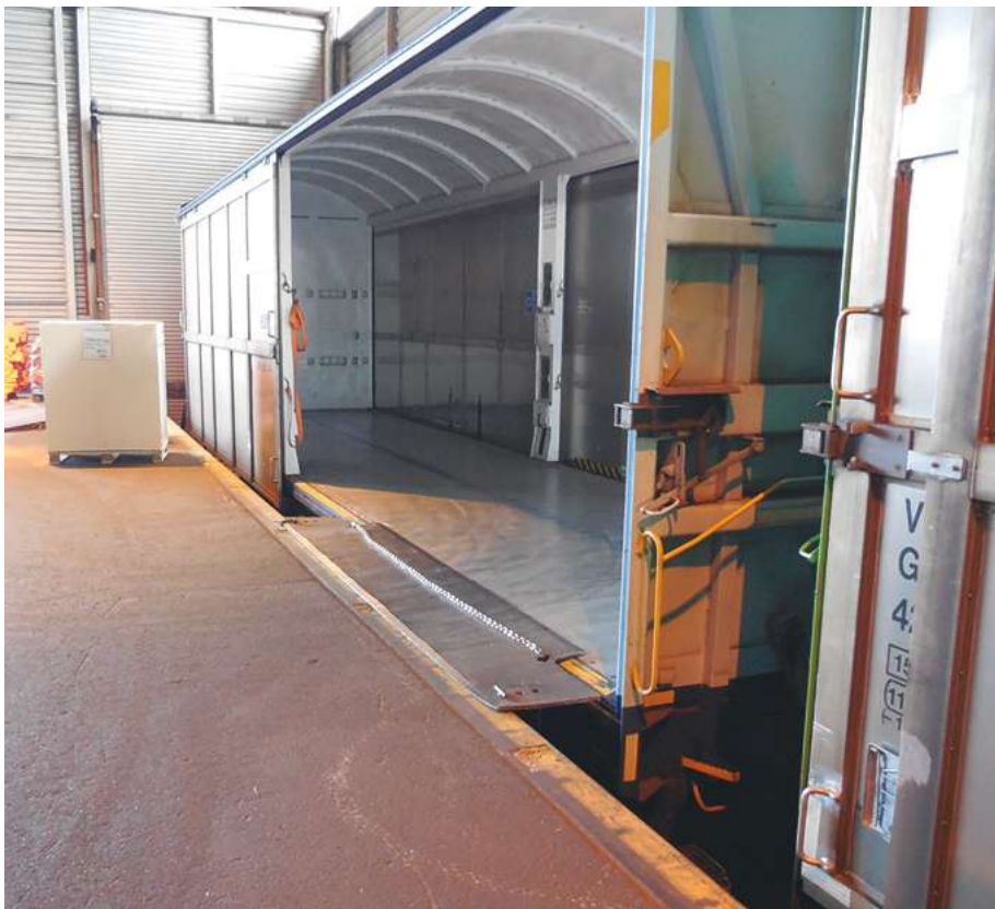
Rail wagon with sliding doors ready for loading. Source: IFP&C
