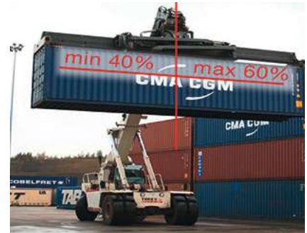
A container load must be balanced correctly to avoid handling difficulties, accidents, and load instability on a carrier. A rule of thumb is to ensure that cargo weight is distributed within a 60-40 % ratio around the centre of the container. Source: Holmen
