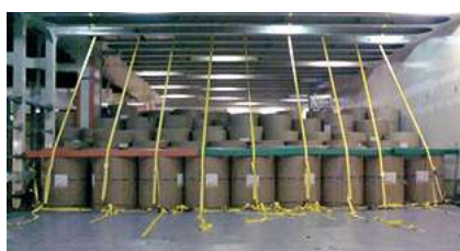
Step-down securing of StoRo cargo. Source: Stota-Enso
