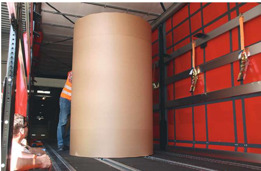
Joloda trailer with rail loading, steel wedges and lashing systems provide optimised securing, transport and handling of paper. Source UPM
