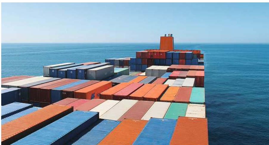
Containers exposed to the sun can have temperature variations of 20-30°C (68-86°F). Any moisture trapped inside will evaporate and when the temperature falls at night condenses and drops onto the paper cargo. Source: Hapag-Lloyd
