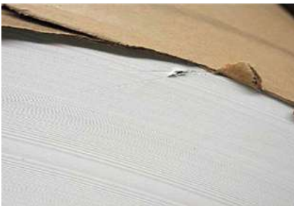
Avoid knife damage to roll. Source: ERA
