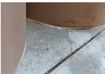
Paper damaged by water leaks. Source: UPM
