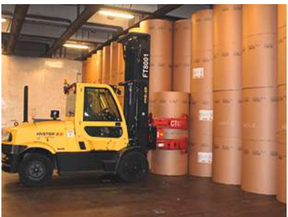
Precise final roll stowing in StoRo hold. Source: Stora Enso
