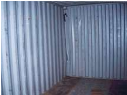
13 Dented internal front panel.
