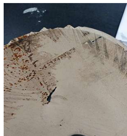
Roll damage from a wet and rusty vessel floor. Source: UPM
