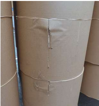
Damage due to sharp clamp pad edge. Source: UPM
