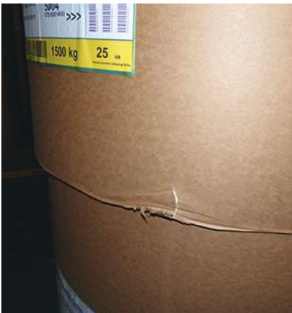
Edge damage from overlapping rolls. Source: UPM
