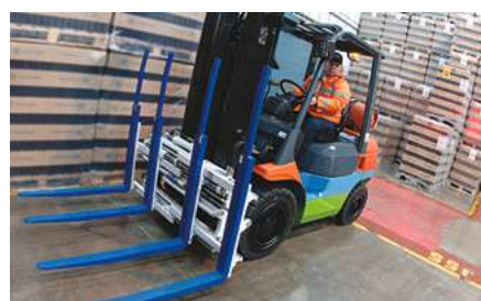
Fork positioners are the most suitable solution to handle pallets of sheet paper because they can be adapted easily to different pallet sizes. Source: KAUP
