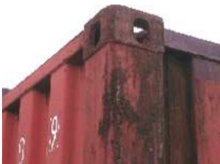
30 Upper corner castings lifting point.
