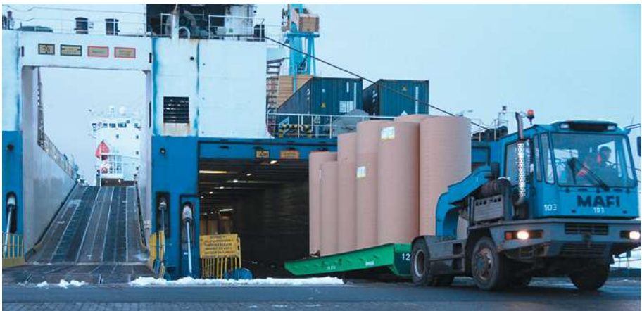
Rolls on a trailer being towed off the ship by a MAFI tug master (tractor). Source INTAKT
