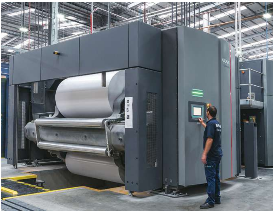
Flying splicer pastes at full production speed. Source: Goss
