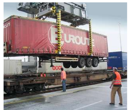
Combi road trailer on rail wagon. This photo shows two bad safety practices: (1) staff not wearing hard hats, (2) a person under a suspended load. Source: INTAKT
