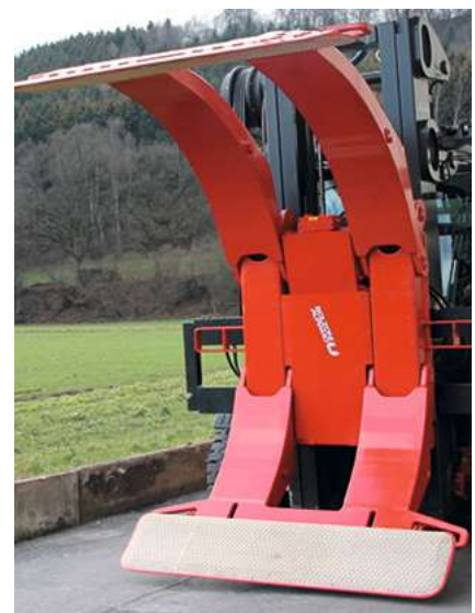
Special clamps are used to handle large diameter tissue rolls. Sources: Bolzoni Auramo
