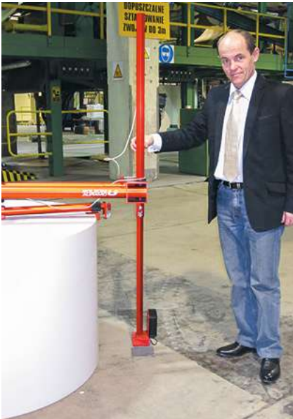
An out-of-round measuring device. Ultrasonic technology can be used to quickly and accurately measure roll roundness without disturbing its wrapping. The results can be viewed on an LCD display and exported to a data management system. Note, this photo shows bad practice of a person in a work area not wearing safety equipment. Source: Bolzoni Auramo
