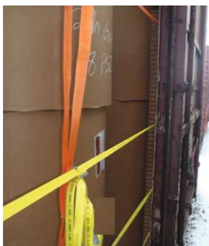
Rolls damaged from door posts. Source: Idealliance
