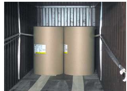
Lashing belts must be prepared and lashed to the container before loading the last rolls. Source: UPM
