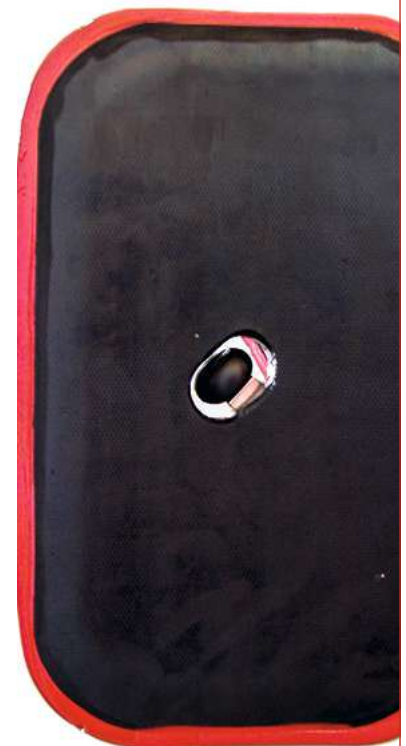
Electronic slip sensors are mounted on the long arm contact pads to measure the paper roll movement in relation to the contact pads. Source: Bolzoni-Auramo
