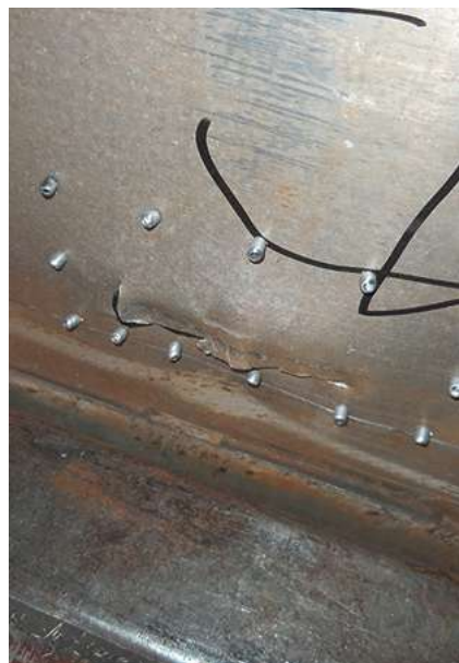
Poor repair of a rail wagon. Source IF P&C
