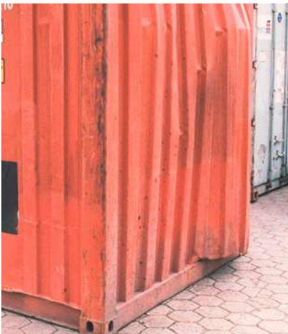
Container wall damaged by the cargo within. Source: FMS 'Use No Hooks'
