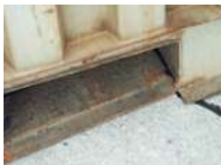
22 Cracked forklift pockets.
