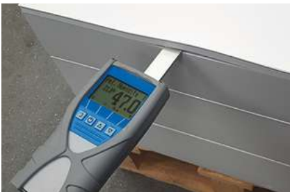
Relative humidity in a paper pile can be measured with a sword gauge. Source: Stora Enso
