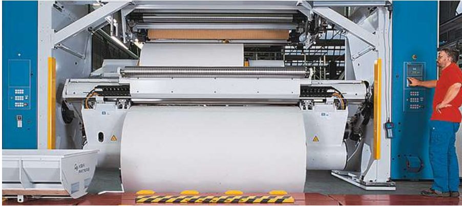
Flying splicers for heavy and wide rolls are equipped with automatic loading. This can include a core container (left) into which the expired roll can be placed. Source: KBA
