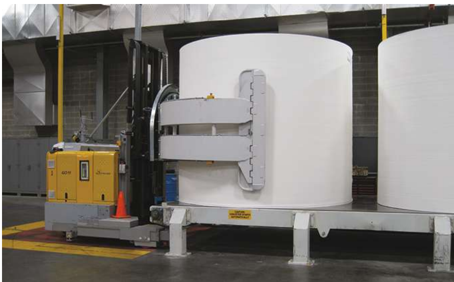
Special clamps are used to handle large diameter tissue rolls. Sources: Cascade
