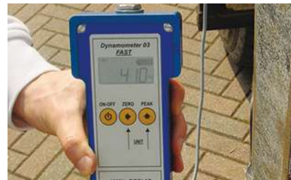
1: A clamping force indicator that displays the clamping force with a calibrated or digital display. Source: Cascade
