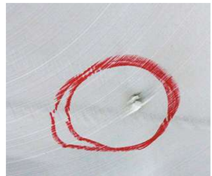
✗ Potential roll end damage source — loose screw. Source: IF P&C
