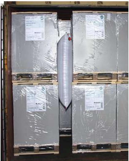
✓ Correctly placed airbags reduce damage by preventing cargo moving into gaps. Air bags inflated to their specifications are relatively hard. Source: INTAKT
