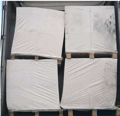
Cargo shifted into voids. Source: Mëtsa Board
