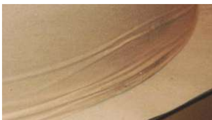
Crimped edge/elephant toes. Source: Stora Enso
