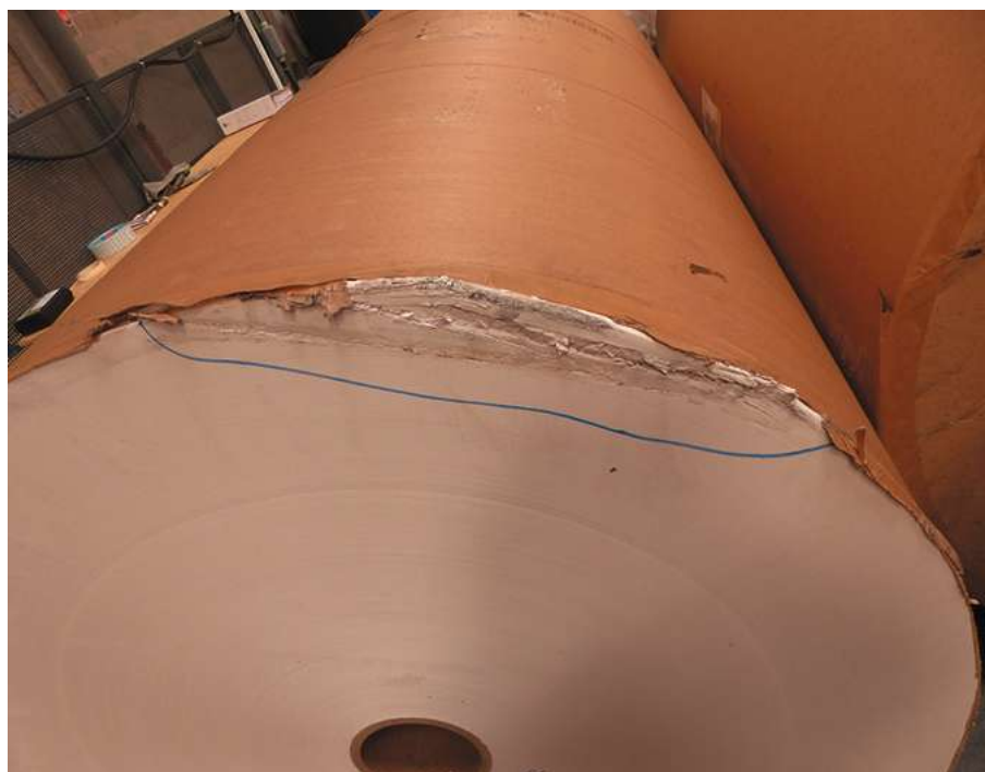
End damage from poor handling. Source: UPM
