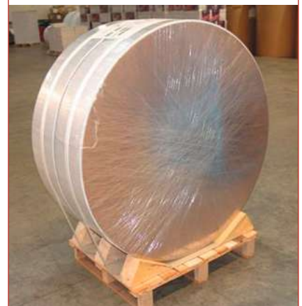
Standing roll loaded on to a pallet and securely chocked both sides. Source: UPM
