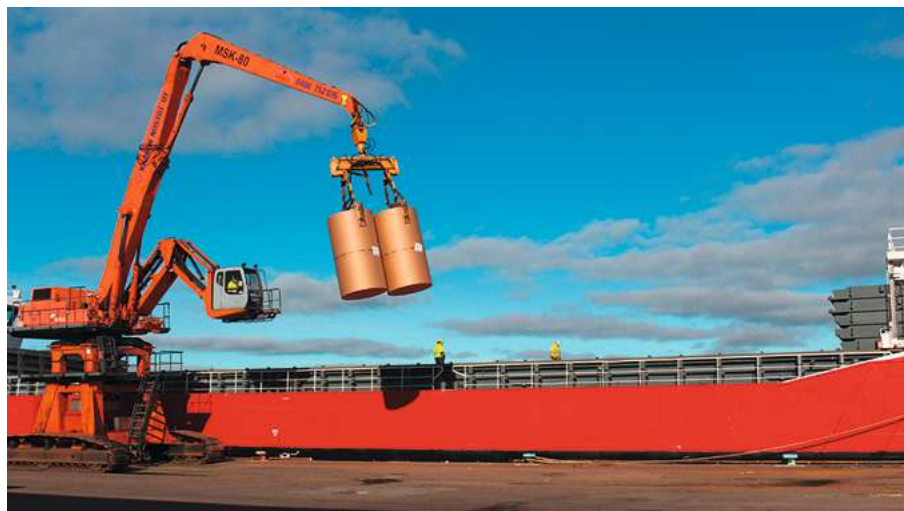
LoLo operation by Mantsinen. A mobile hydraulic crane equipped with clamps for roll loading. Source: Stora Enso
