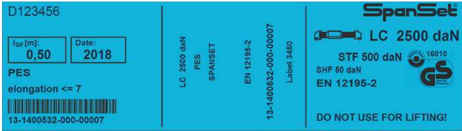
Lashing belts must carry a rectangular, long lasting rating label containing all performance specifications for the lashing. Source: SpanSet
